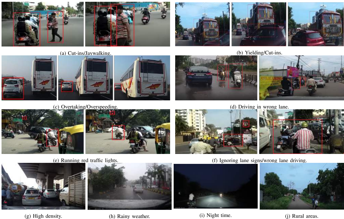
Fig. 2: Annotations for rare instances: One of the unique aspects of METEOR is the availability of explicit labels for rare and interesting instances including atypical interactions, traffic violations, and diverse scenarios. These annotations can be used to benchmark new methods for object detection and multi-agent behavior prediction.
