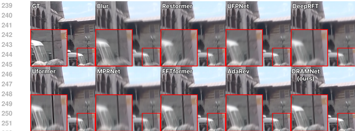
Figure 4: Comparison of deblurring results from various methods on one of the more challenging examples from GoPro dataset, including DRAMNet and AdaRevD-L. The bigger red-highlighted region is a zoomed-in crop taken from a smaller area to clearly illustrate the differences.
