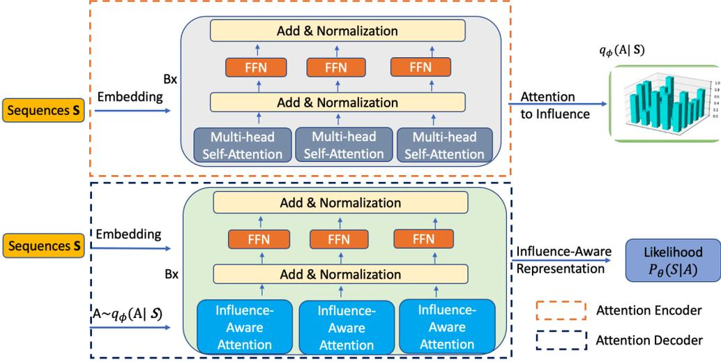
Figure 1: Neural architecture of IAA-MTPP. The attention encoder takes an event sequence  $S$  and outputs an approximate posterior  $q_\phi(\mathbf{A}|S)$  of latent relation; the attention decoder takes the same sequence and a sample  $A$  from  $q_\phi(\mathbf{A}|S)$  and outputs a influence-aware high level representation to be used for modeling the likelihood given influencing matrix  $A$ .
