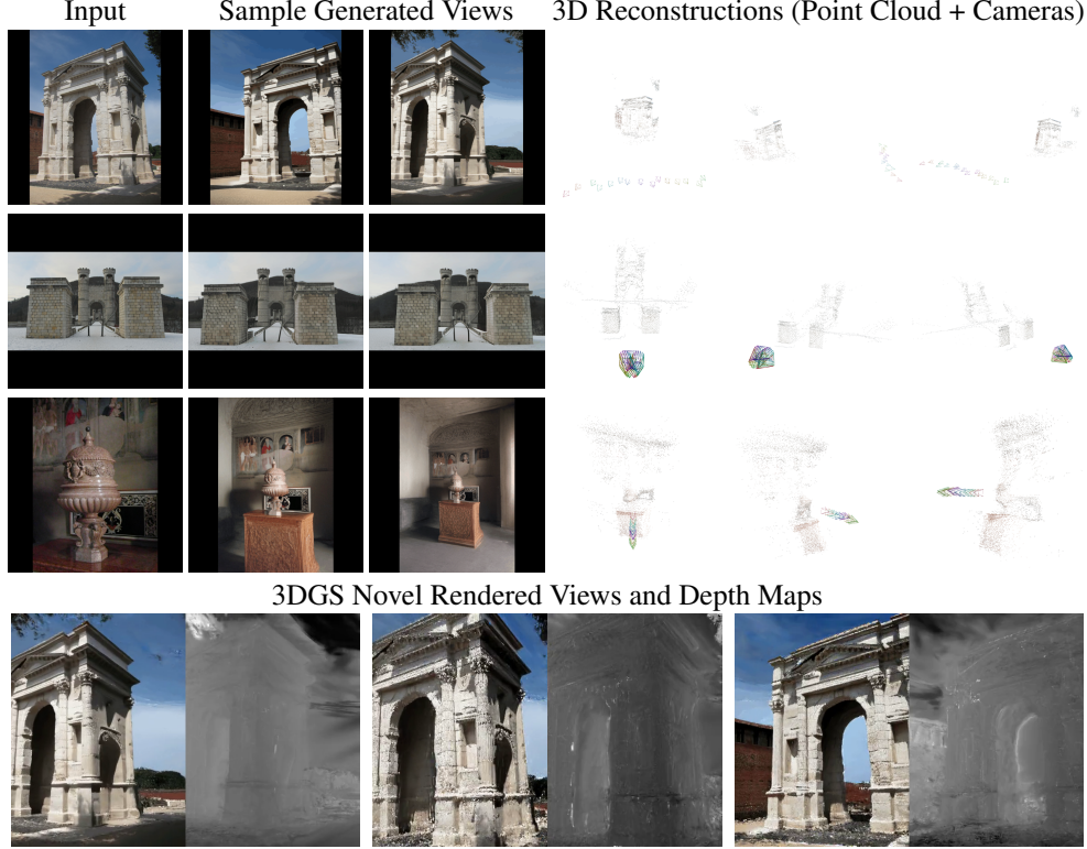
Figure 10: 3D Reconstruction from Generated Views. We show 3D reconstruction results applied to WildCAT3D generations, as described in Appendix A.4. Reconstructed point clouds and camera positions are shown above, generally matching the expected scene geometry and camera trajectories used for generation. While two generated views are shown for conciseness, 3D reconstruction results are calculated from 15 views. We also show an example of novel views and their normalized depth maps generated using a 3D Gaussian Splatting (3DGS) representation initialized with the sparse reconstruction of the first scene.
