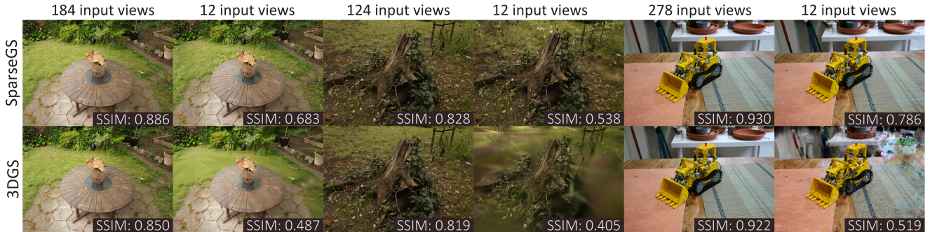
Figure 1. The quality of 3DGS [11] degrades as the number of input views decreases , particularly in unbounded scenes. SparseGS significantly improves novel view synthesis quality in sparse-input settings while maintaining fast training and real-time rendering.
