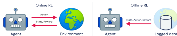
Figure 1: In online RL (left), the agent must interact with the environment to gather data to learn from. In offline RL (right), the agent must learn from a logged dataset.
