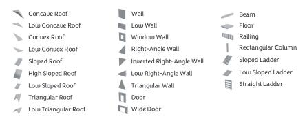
Figure 8: **Descriptions of primitives in building data.** We showcases roof primitives, wall primitives, and other component primitives in three columns.
