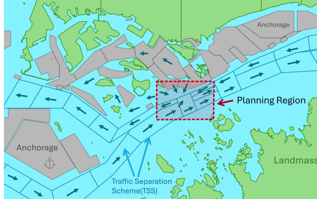
Figure 3: The red region is used as the environment area. The gray areas indicate anchorage zones, the green areas represent landmasses, and the arrows and regions with dark blue borders represent the Maritime Traffic Separation Scheme (TSS). The high density of crossing points in the red area makes it a more challenging region for navigation, providing a suitable setting for testing advanced planning techniques.
