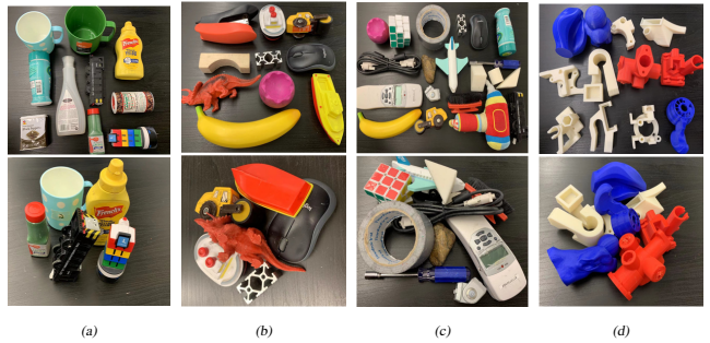
Fig. 7. Object sets and test configurations used for real robot experiments. From left column to right column: packed scene with 10 objects; pile scene with 10 objects; 20 test hard objects [31]; 12 Berkeley adversarial objects [16].
