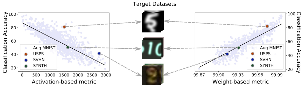
Figure 1: Correlation between classification accuracy and different metrics: Pearson correlation between network weights (right, our method) and Fréchet distance between network activations (left, (Deng & Zheng, 2021)). Note that our method yields a more reliable performance estimator, as evidenced by the points corresponding to the target datasets lying closer to the black line. The light-blue points correspond to sample sets from the meta-dataset.
