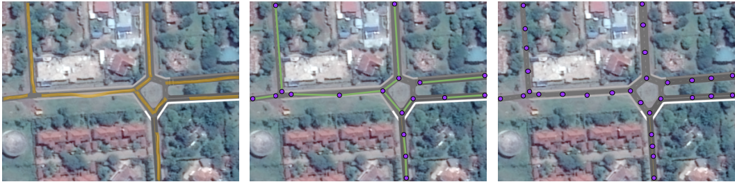
Figure 15: Example of how key points are generated. We start by evaluating a segmentation model (left) and extracting the predicted graph (middle). We then over-sample vertices along edges to enlarge the action space (right).
