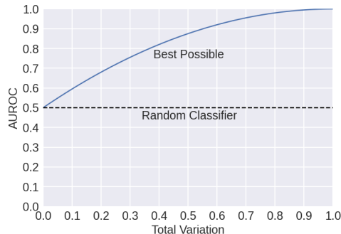
Figure 8: Comparing the performance, in terms of AUROC, of the best possible detector to that of the baseline performance corresponding to a random classifier.
