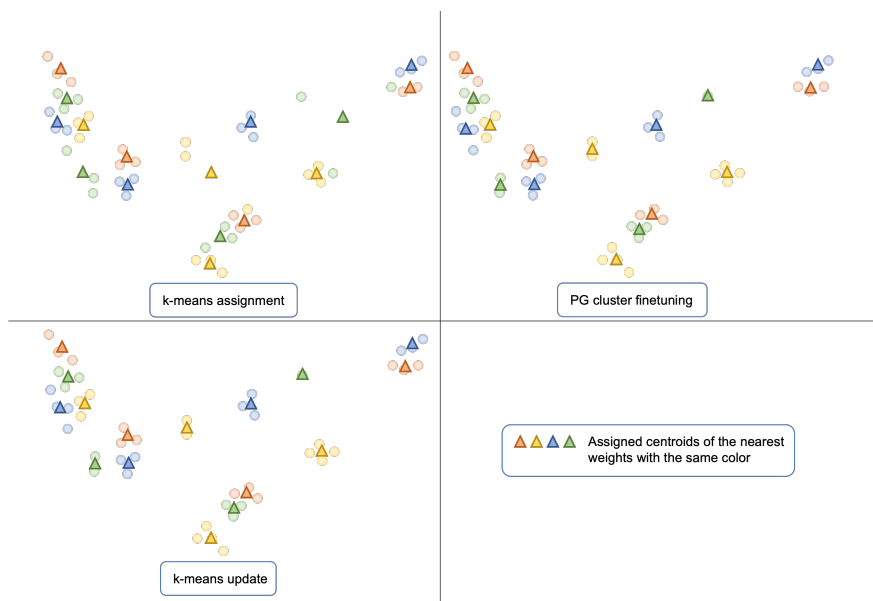
Figure 6: Illustration of complete PG k-means method during k-means iterations. With the optional Dense Weights Consolidation step, the number of weights was reduced from 50 to 47, improving our method's ability to represent isolated, small clusters while decreasing the probability of empty clusters.
