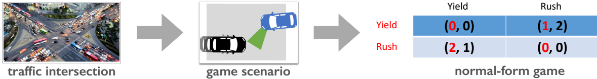
Figure 4: A snapshot of stochastic time in the intersection example. The scenario is abstracted such that there are two cars, with each car taking one of two possible actions: to yield or to rush. The outcome of each joint action pair is represented by a normal-form game, with the reward value for the row player denoted in red and that for the column player denoted in black. The Nash equilibria (NE) of this game are (rush, yield) and (yield, rush). If both cars maximise their own reward selfishly without considering the others, they will end up in an accident.
