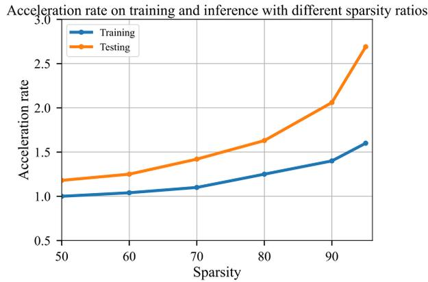
Figure 14: Training and inference acceleration on hardware of ResNet-32 on CIFAR-10.
