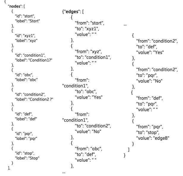
(b) Graph representation in JSON (JavaScript Object Notation) with nodes and edges.
