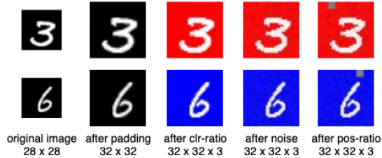
Figure 1: The conversion process used to generate samples. Input image is first padded to become 32x32. The attributes clr-ratio is then applied, which decides the background color (blue or red). Noise is then added to the background color. Finally, pos-ratio affects the positioning of the box (top row, left half or top row, right half). Check Section D of the Supplementary for more details. Best viewed in color.
