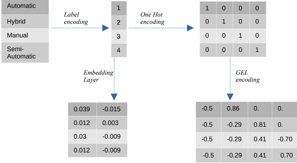
Figure 1: Representation of encodings and embeddings for an example containing four unique values.
