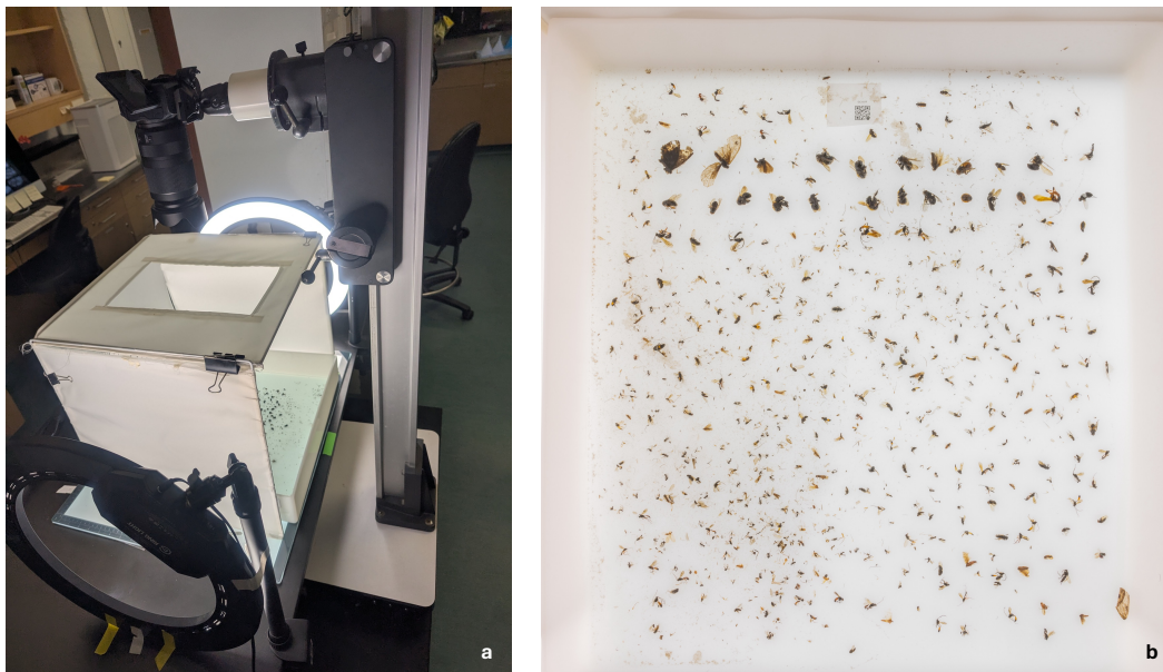
Figure 4: (a) Imaging setup used to capture bulk images of the MassID45 dataset, including the positioning of the camera, light cube and ring light sources. (b) A representative image captured using the described imaging setup, with the sides trimmed, showcasing the high density of the insect specimens. Images are reproduced from [21].
