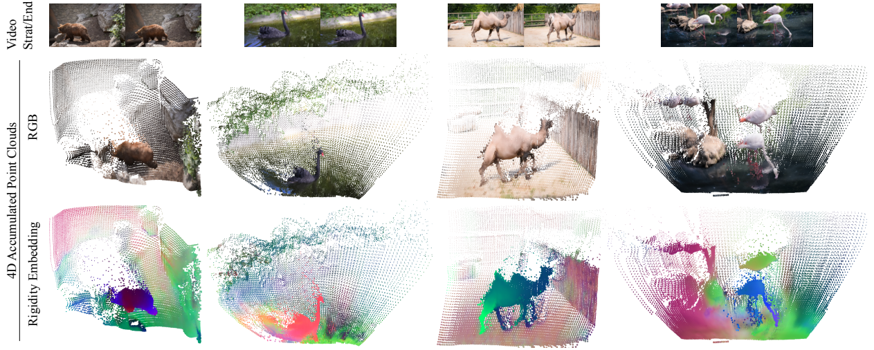
Figure 6: Per-Scene Intermediate 4D Reconstructions Using Off-the-Shelf Depth. While we emphasize that geometry estimation or 4D reconstruction is not the primary aim of our method, here we plot accumulated 4D point clouds and their corresponding unprojected rigidity embeddings after per-scene reconstruction using off-the-shelf monocular depth estimates.
