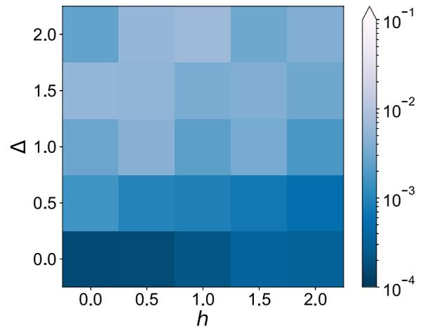
FIG. 13. Relative error of the ground state energy,  $|(E - E_{\text{ground}})/E_{\text{ground}}|$ , after fine-tuning the TQS on specific parameter points for  $2 \times 10^3$  iterations.
