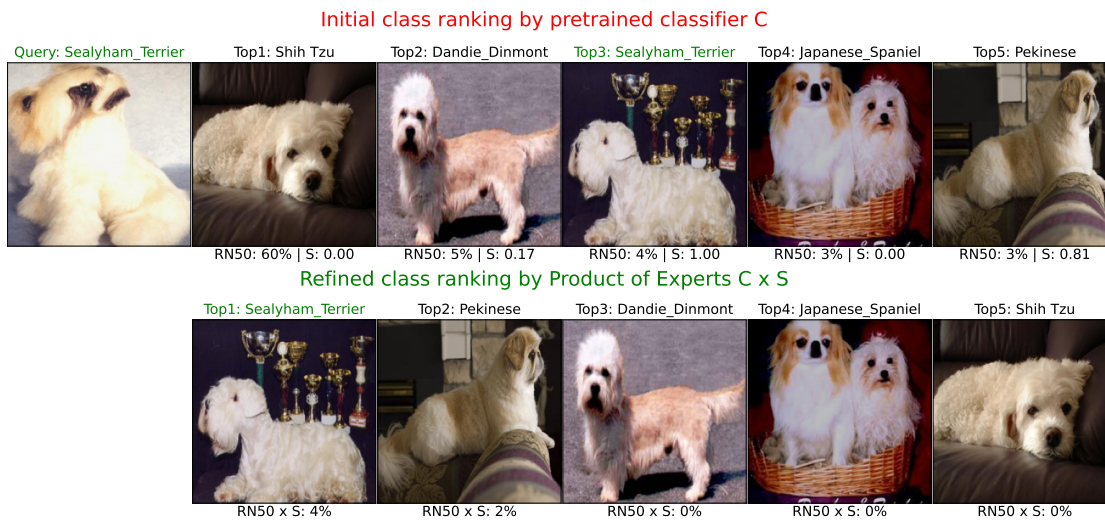
Figure 26: A pretrained model C makes predictions on the Query image (ground-truth label: Sealyham Terrier) and produces initial ranking (top row) but the top-1 predicted class does not match the ground-truth label. The refined class ranking is presented in the bottom row where the Sealyham Terrier class has been recognized as top-1.
