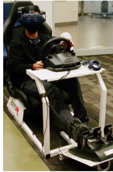
Figure 3: Physical setup with a driver in a driving pose, driving the ego vehicle within the DREyeVR [16] simulator.
