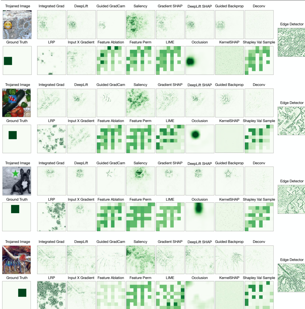
Figure 5: Examples of trojaned images, ground truth attribution maps, and attribution maps from various methods, including an edge detector baseline. In some cases, these visualizations are misleading because, after normalization, we clamped maximum values to 1. This clamping distorts differences between large values. See Figure 6 for quantitative results.
