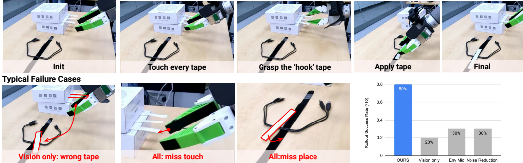
Fig 6: Taping Evaluation. In the first row, we show the task definition. The second row shows the typical failure case for each method and the overall task success rate.
