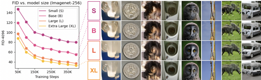
Figure 5: One-step generation quality continues to improve as model parameter count increases. While generative models tend to display continual improvement with model scale, bootstrap-based methods such as Q-learning have been shown to lose this property (Kumar et al., 2020). We show that shortcut models, while a bootstrap-based method, retains the ability to scale accuracy with model size.
