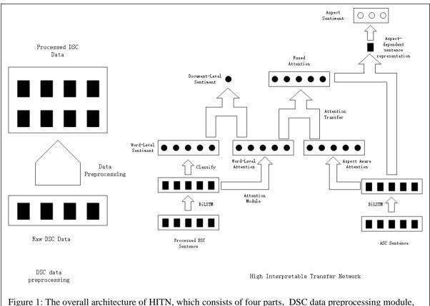
Figure 1: The overall architecture of HITN, which consists of four parts, DSC data preprocessing module, pre-trained DSC module, ASC module, and attention transfer module.
