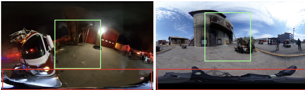
Figure 7: Illustration of distortion severity in Fire360 equirectangular projections. Green regions exhibit minimal distortion, preserving the geometric structure, while red regions show significant stretching at vertical extremes, degrading localization, and retrieval accuracy.
