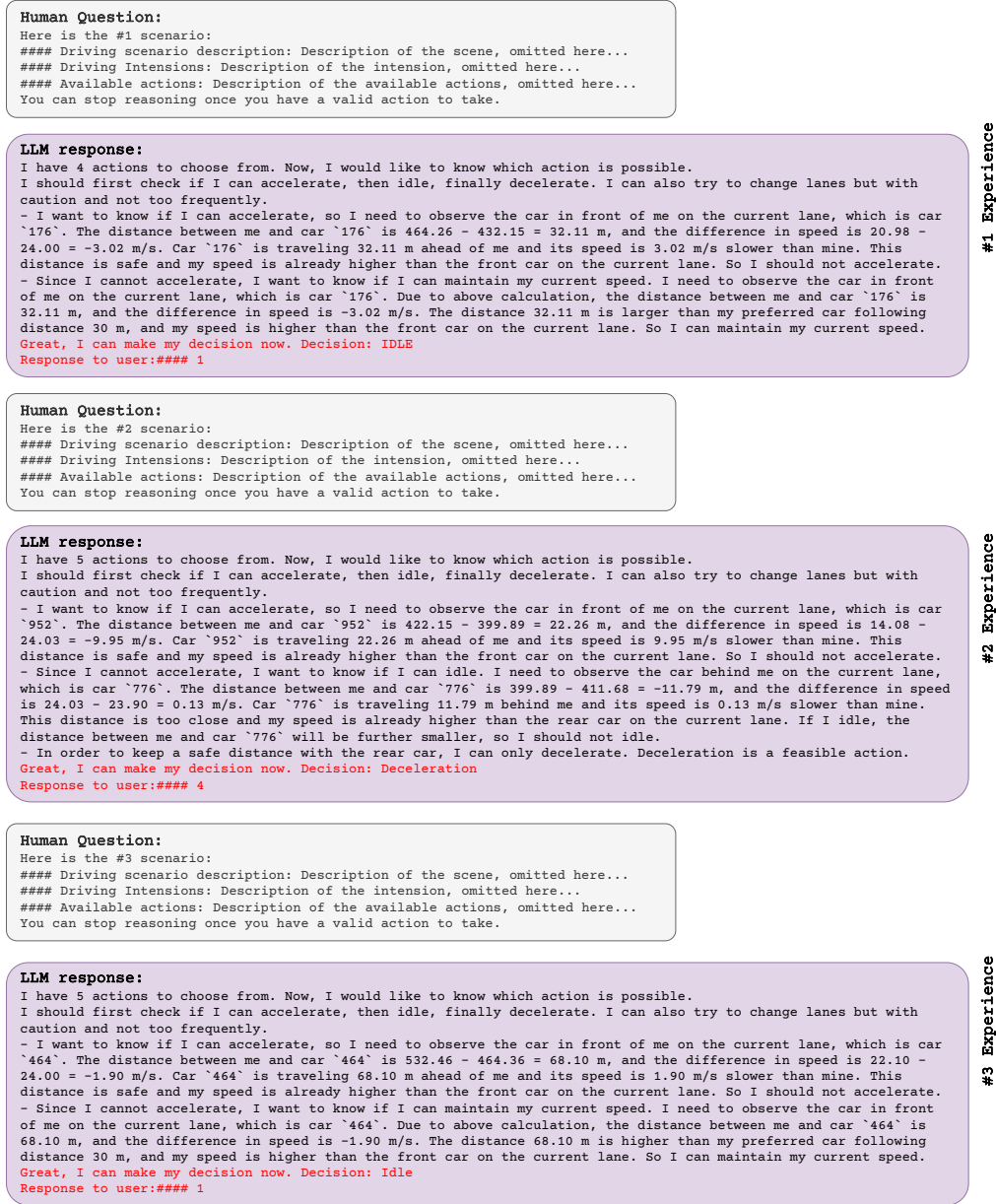
Figure 8: The 3-shot prompts example for the scenario shown in Figure 7. DiLu recall top three most similar experience from the memory module which contains 2 idle and 1 deceleration decision. The few-shot experience is entered into GPT-3.5 as a "human-LLM" dialogue.
