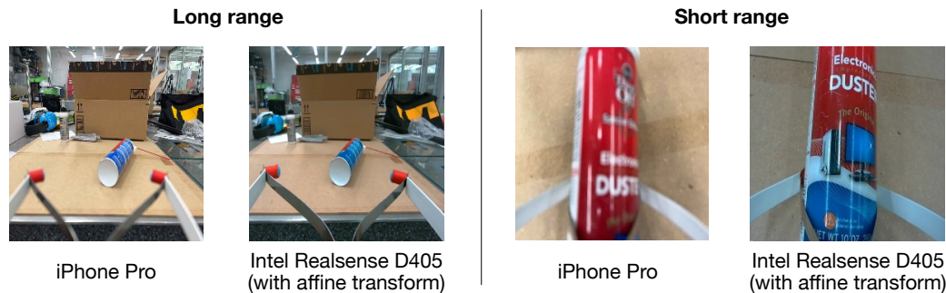
Figure 15: We can see the corresponding D405 camera image alongside the iPhone Pro image. While in the long range, the images look similar, in the short range iPhone images are out of focus because of the different focal lengths of the cameras.
