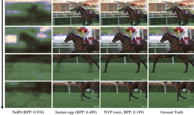
Figure 1: Reconstruction results on Jockey in UVG-HD after training each model for “1 minute” with a single NVIDIA V100 32GB GPU. NVP can capture the detail of a video containing dynamic motions, e.g. , the legs of a running horse, while the prior methods generate blurry artifacts.
