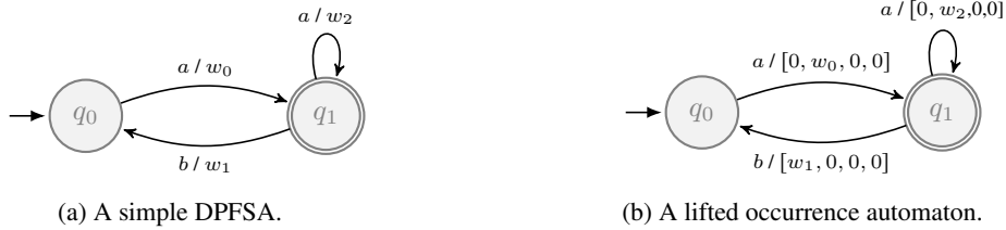
Figure 2: The lifted occurrence automaton is on the right, with the original automaton to the left. We target the symbol a for four occurrences. q_0 is the starting state and q_1 the accepting state.
