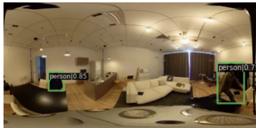
Figure 8: An example of object detection results. While the object detector detects people, the detector does not detect a sink, which is slightly to the right of the center.
