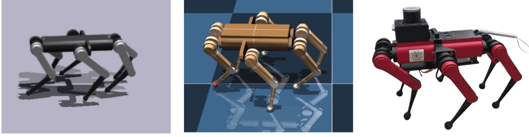
Figure 10: Custom-built hexapod robot in Isaac Gym, MuJoCo, and the real world.
