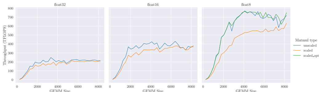
Figure 22: Square matrix multiplication throughput in TFLOPs with and without scaling factors applied to the output across 32-, 16-, and 8-bit float dtypes on NVIDIA H100 PCIe. Naive implementation in PyTorch.
