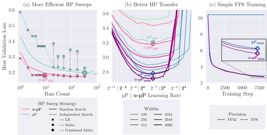
Figure 1: (a) Two different HP sweeping processes used for \mu P and u- \mu P proxy models. Unlike \mu P, u- \mu P admits independent (1D) search due to careful HP design. The first part of independent search is an LR sweep, which alone reaches near-optimal loss for u- \mu P. (b) Using the best proxy HPs from (a), we train many models at different widths and LRs. The best LR for width 256 is \sim optimal for 4096, showing LR transfer along with lower loss. (c) We re-train with a simple un-scaled to(float8) cast on matmul inputs. This would fail for other models, but u- \mu P trains with minimal degradation.
