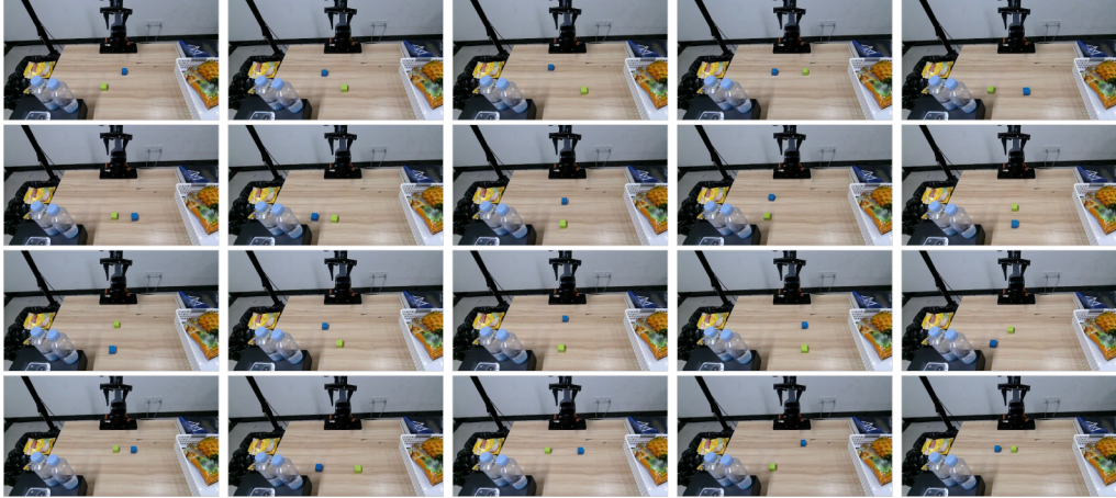
Figure 8: We conduct 20 trials for each real-world task, randomizing the task configurations in every trial. The language command for this task is “stack the green cube on the yellow cube.”
