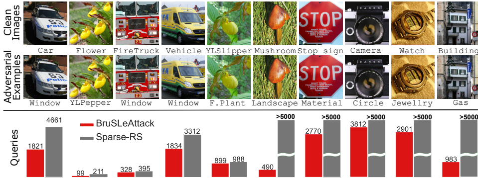
Figure 6: Demonstration of sparse attacks against GCV in targeted settings with a budget of 5K queries and sparsity of 0.5% \approx \frac{250}{224 \times 224} . BRUSLEATTACK can yield adversarial examples for all clean images with less queries than SPARSE-RS while SPARSE-RS fails to yield adversarial examples for Mushroom, Camera, Watch, & Building images. Illustration on GCV API (online platform) is shown in Appendix Q.
