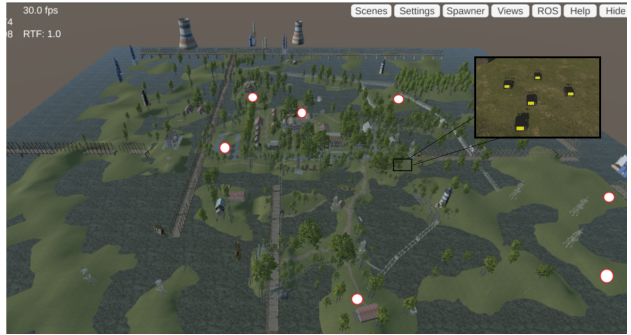
Fig. 1. A multi-robot team is deployed in a simulated environment to search for targets of interest (represented by white points). Effective teammate-aware active search will enable the robot team to identify targets while maintaining communication with teammates.
