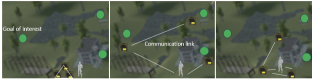
Fig. 3. The progression of a multi-robot team during a teammate-aware active search mission. Frame 1 shows the robots starting together, ready to begin their search. In Frame 2, the robots split up to explore multiple targets. Frame 3 illustrates the robots maintaining communication while spread out, ensuring they stay connected.
