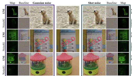
Figure 5: Gaussian and shot noise create visual artifacts prominent in noised-baseline IG. Frequency bias leads to disparate scores for adjacent pixels.
