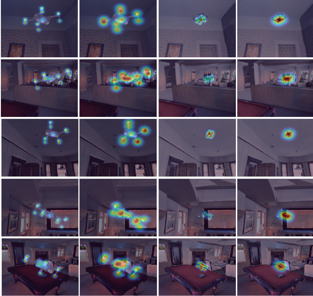
Figure 2: Qualitative heatmap results on random samples from the test-set. The first two columns depicts the M2ED drone while the last two the Tello drone; with heatmaps predicted by models trained with l_p and l_h respectively. Evidently, heatmaps by the l_h model ( second and fourth columns tend to keep the 2D Gaussian shape distribution, while the l_p ones ( first and third columns ) freely approximate the (x, y) position enforced by the regularizer term ( l_{reg} ) of the l_p loss, eventually allowing for more distinguishable 2D keypoints estimations.
