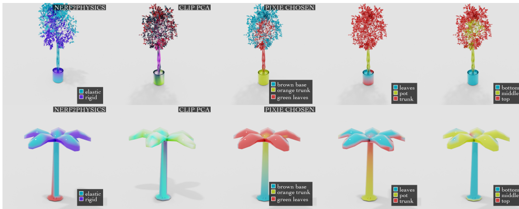
Figure 10: CLIP Semantic Segmentation. CLIP features can be noisy for various objects and different text queries vary greatly in segmentation quality. Thus, we prompt a VLM actor to generate several candidate queries for each object, render all candidates, and prompt another VLM critic to select the best query terms from the rendered 3D segmentation images. Some candidates are provided and proposals chosen by the critic are highlighted. Note that a high-performing query proposal (e.g., “leaves,pot,trunk”) in one object is not necessary high-performant in another. The PCA visualization of the CLIP feature fields is also provided.
