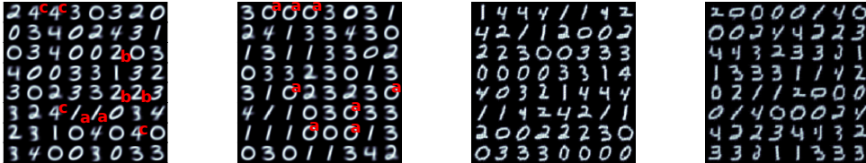
Figure 4: Sampling diversity: top-1 sampling shown on MNIST, from left to right, for DCGMM architectures 1L (vanilla GMM), 2L-d (non-convolutional 2-layer), 2L-c and 2L-e (convolutional 2-layer). Please observe duplicated samples in the non-convolutional architectures, marked in red.
