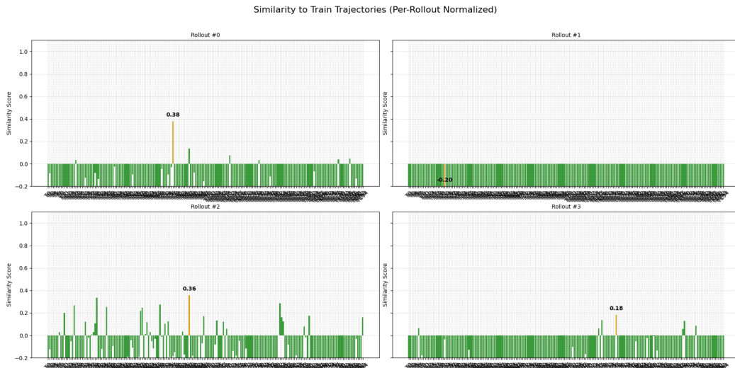
Figure 23: Analysis of a Diffusion Policy model roll-outs on training set with respect to all ground-truth training trajectories. The model was trained on the “Square” benchmark.
