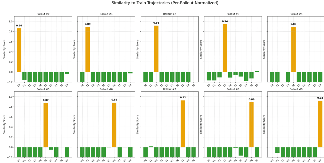
Figure 16: A subset of the total analysis done for the roll-outs of a Diffusion Policy model from the training set with respect to all ground-truth training trajectories. The model was trained on the “Can” pickup benchmark.
