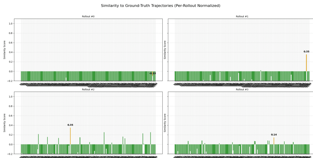
Figure 19: Analysis of a Diffusion Policy model roll-outs on the validation set with respect to the ground-truth training trajectories. The model was trained on the “Can” pickup benchmark.
