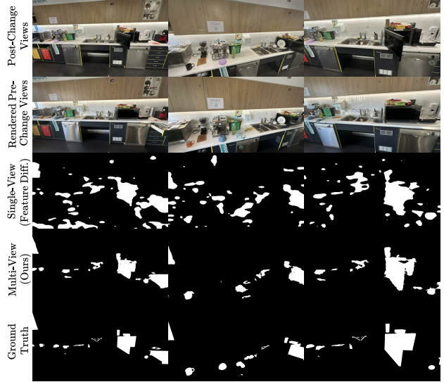
Figure 1. Our multi-view approach to visual change detection (second row from bottom) enforces consistency of the predicted changes across multiple viewpoints by embedding change information in a 3D Gaussian Splatting model of the scene. This effectively suppresses many of the false-positive detections exhibited by current single-view methods (middle row).
