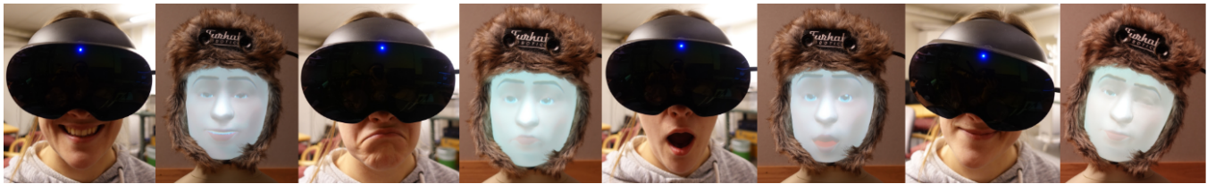
Figure 3: Face tracking with a VR headset displayed on Furhat’s face mask showing the operator’s face and the corresponding facial expression on the robot.
