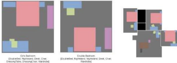
Fig. 7: Sample outputs of the population stage. Left, Center : Single-room inference for a given room type and a list of objects. The objects are placed in an intuitive way that allows humans to interact with objects in a realistic way. Right : Result of population stage applied to an entire residential floorplan. Different room types (bedrooms, living room) are populated alongside each other. The object positioning takes doorways into account and leaves walking space in every room.
