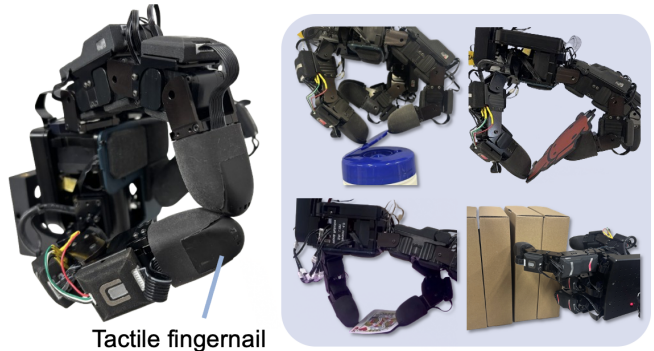
Fig. 1: We extend a conventional uSkin fingertip with a 6D force-torque sensorized tactile fingernail, enabling nail-assisted interactions such as edge engagement, peeling, scraping, and thin-object manipulation.
