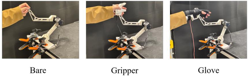
Fig. 2: Overview of the ACE-F system. **Left:** Annotated view of the ACE-F arm showing the base joint (1 DoF), perpendicular elbow joints (2 DoF), and the magnetic spherical joint for interchangeable end-effectors. **Right:** Three representative end-effector configurations are enabled by the spherical joint, using a bare setup, gripper attachment, or wearable glove.
