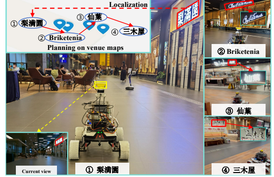
Fig. 1: We propose to leverage the textual information in a venue map to facilitate shop searching in unknown open-world environments. The robot localizes itself in the environment by recognizing and matching the texts on a sign to the venue map. Then the robot plans a direction to the next landmark ‘Briketenia’.
