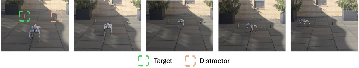
Figure 5: Example run of the Unitree Go2 robot performing an object-finding task using vision-language-based control. The robot receives the instruction “ find the silver bottle ” and navigates the environment while distinguishing the correct object from a similar distractor.
